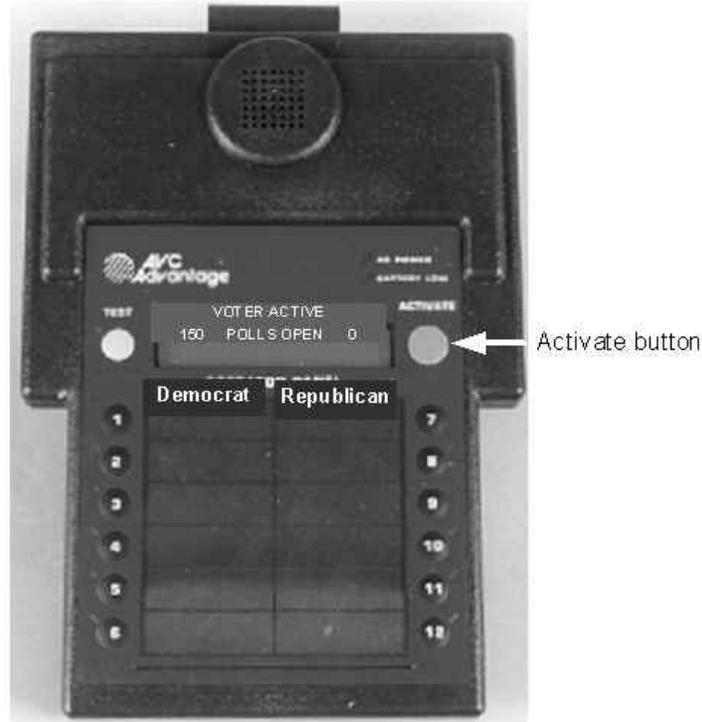
Figure 18. Operator Panel – Activate
